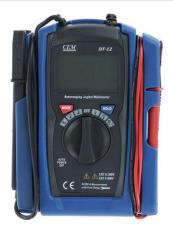
4000 counts, 8 functions including DCV, ACV, DCA, ACA, Resistance, Continuity, Diode test with Data Hold, Low impedance and non-contact ACV detection. Large high contrast 4000 counts LCD display with Analog barograph Auto Power off Relative, and Data Hold Built-in storage compartment for integrated test leads Over-range and low battery indication
